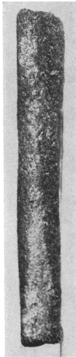
Fig. 4. Cross section of a carbon felt matrix after washing in water showing a zone of unreduced sulphur in the interior.
